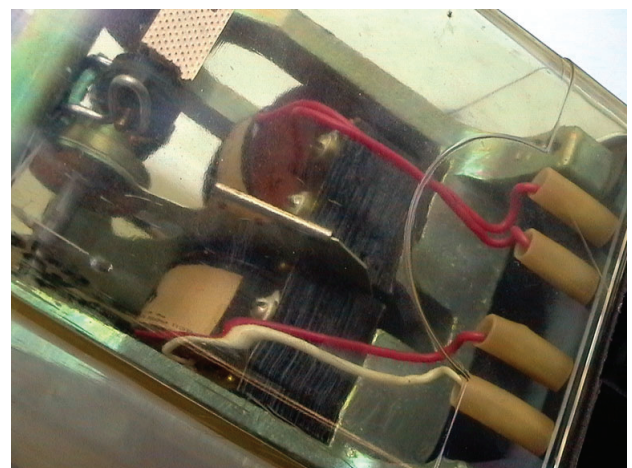
Fig. 2 Phase sensitive relay DSS-12
