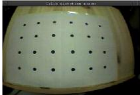
Fig.5. Marker with 6x4 pointsfor calibration
