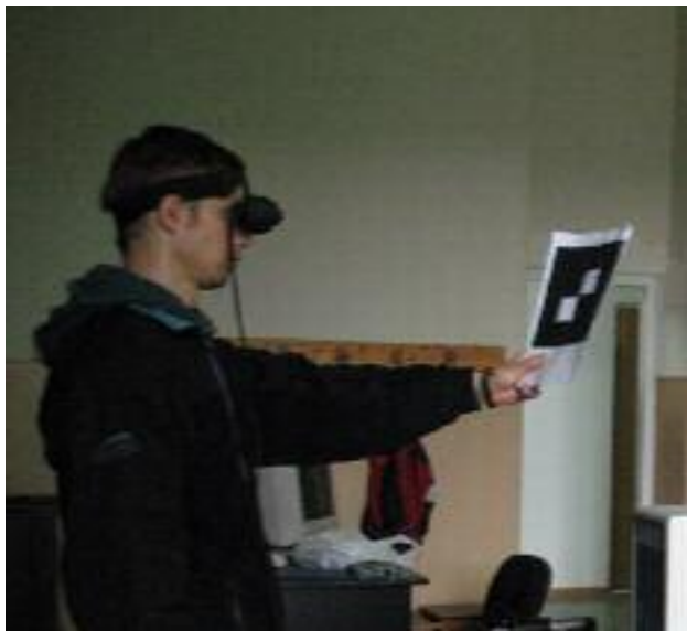
Fig.4. The shape of marker and the position of user when calibrate the video system TriVisio
