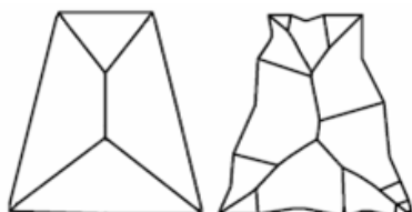
Fig. 2. Sensitivity of skeleton to insignificant boundary changes
