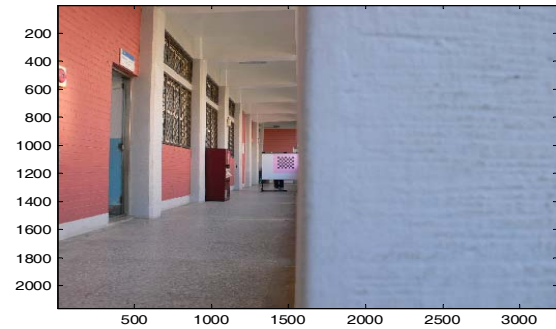
Fig. 10 Measurement of an object at a distance of 1406 cm.
