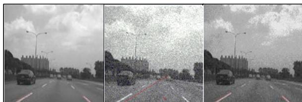
Fig.8 Processing result for lane detection flow and each step images with generic Gaussian 2-D filter and resizing the grouping mask to 9 \times 11 .
