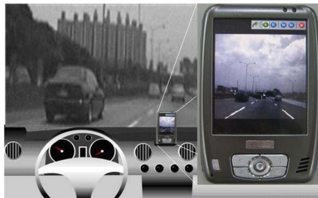
Fig.10 Result for lane detection using Pocket PC with Xscale270 CPU as the platform
