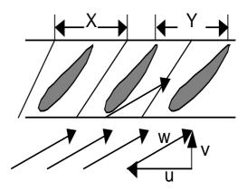
Fig. 6. Illustration of blade row of axial flow pump.
