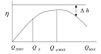
Fig.3 Illustration of overall pump efficiency curve.
