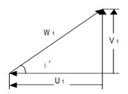
Fig.2 Velocity triangle at impeller inlet.
