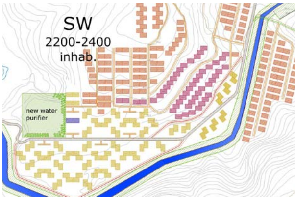
FIG. 4: South-Western new residential zone with new water purifier
