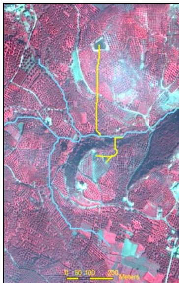
Fig.5. Flow-paths of OMWW from waste tanks to the drainage network.
