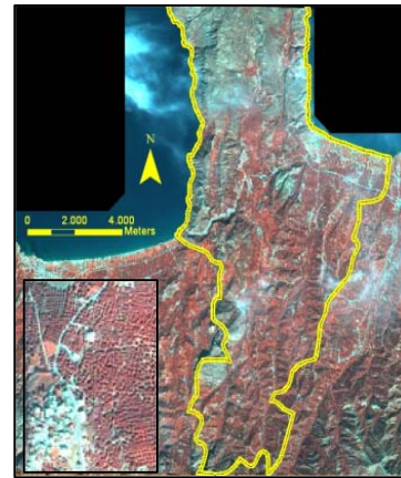
Fig.3. A QuickBird image of the area after implementation of the fusion technique. A close view is shown in the inset.
