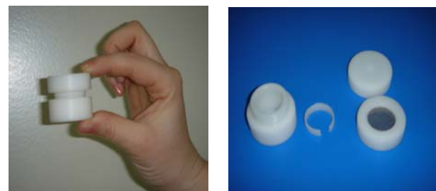
Fig.1. Plastic passive sampler and its parts
