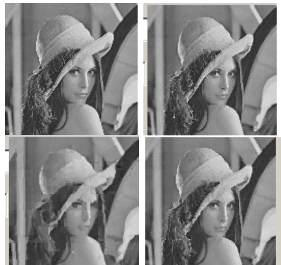
Fig.3 Examples of the reconstructed images: original image(top-left), reconstructed image Jacquin method range 4*4 (top-right), reconstructed image our method range 4*4(bottom-left), reconstructed image our method range 2*2 (bottom-right).
