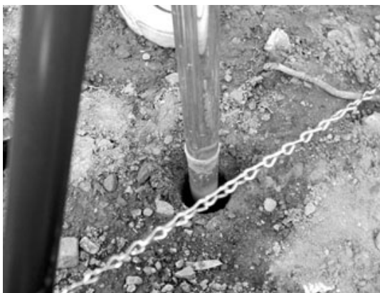
Fig. 2. (a) The equipment of Guelph Permeameter 2800K1 was used in this study.
