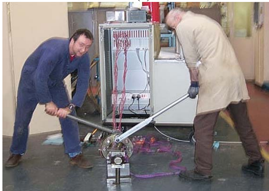
Figure 3: (a) Bolt tightening sequence, (b) Gasketed Flange Joint Tightening
