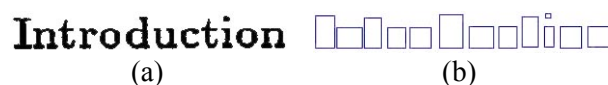
Fig. 4. Characters are represented by rectangles (a) Original image, (b) Rectangle of characters
