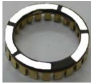
Fig.12. Prototyped vibrator of the 9[mm] outer diameter RUSM.
