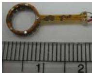
Fig.14. Prototyped flexible PCB for an electric source transmission.
