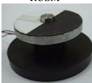
(a) Assembled mechanical system of the 8.5 [mm] outer diameter RUSM Fig.15. Prototyped mechanical system of the proposed RUSM
