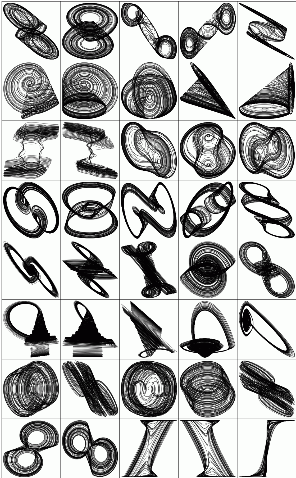
Fig.2: The plane projections of strange attractors modeled by the universal RC oscillator.
