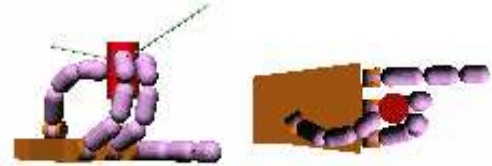
Fig. 10 : Cylinder grasp synthesis using GAs and manipulability maximization
