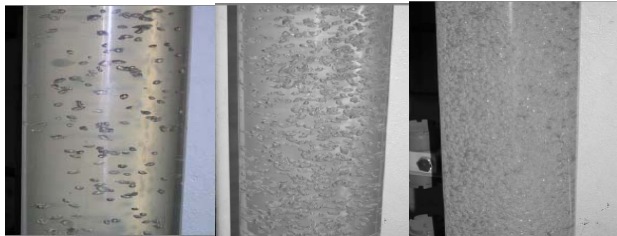
(a) Bubbly flow (b) Annular flow (c) Churn flow Fig.1. Illustration of three different flow regimes
