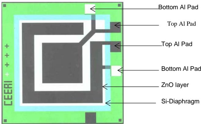
**Fig. 1 Layout of the acoustic sensor**
