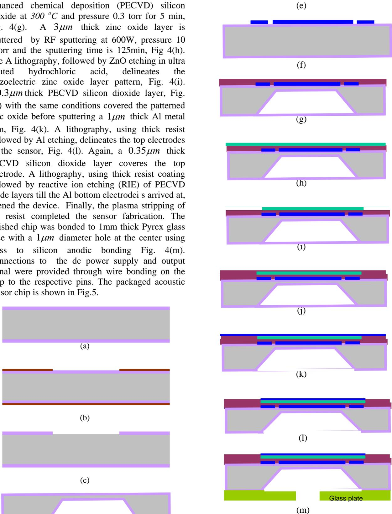
Fig.4 Fabrication and process flow of the acoustic sensor
