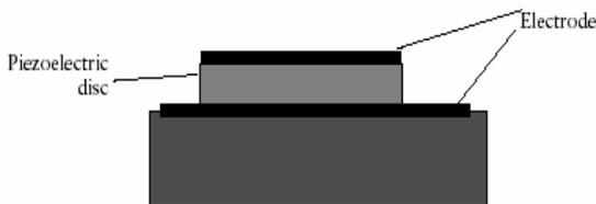
**Fig. 2 Piezoelectric sensing**
