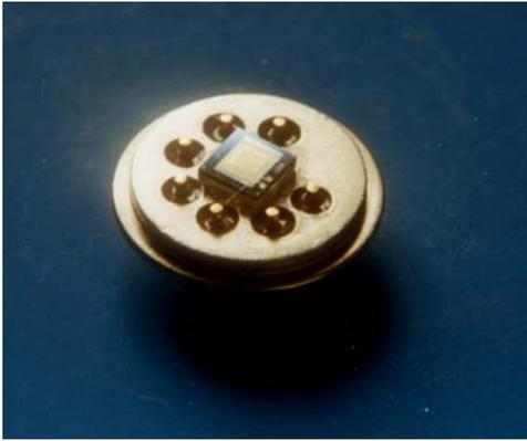
Fig. 5 MEMS based acoustic sensor chip
