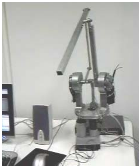
Fig.18. Implementation of 5-barlinkage in the lab
