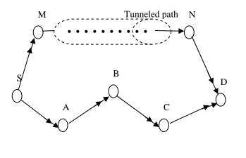
S: source node D: destination node M, N: malicious node A, B, C: intermediate node
