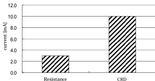
Fig.7. Current that flows to LED
