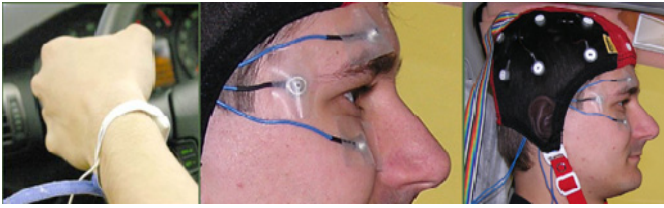
Figure 2: The tested driver equipped with heart beat recording, EOG electrodes and the EEG cap
