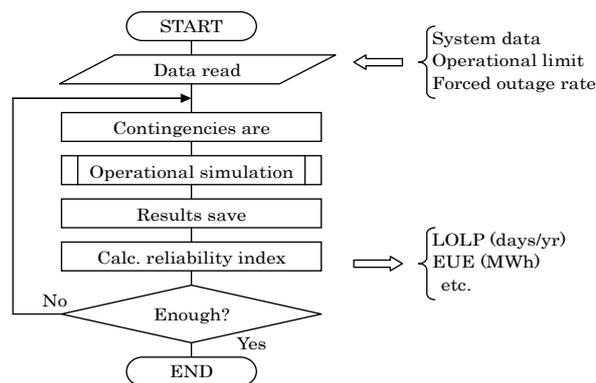
Fig. 1 Flow for Conventional Monte Carlo Method
