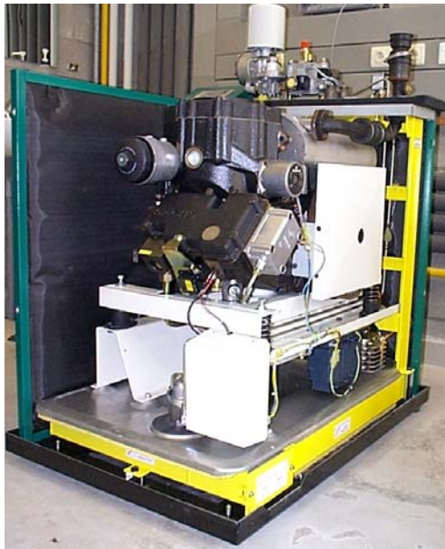
Fig. 4: Picture of the CHP without sound insulation
