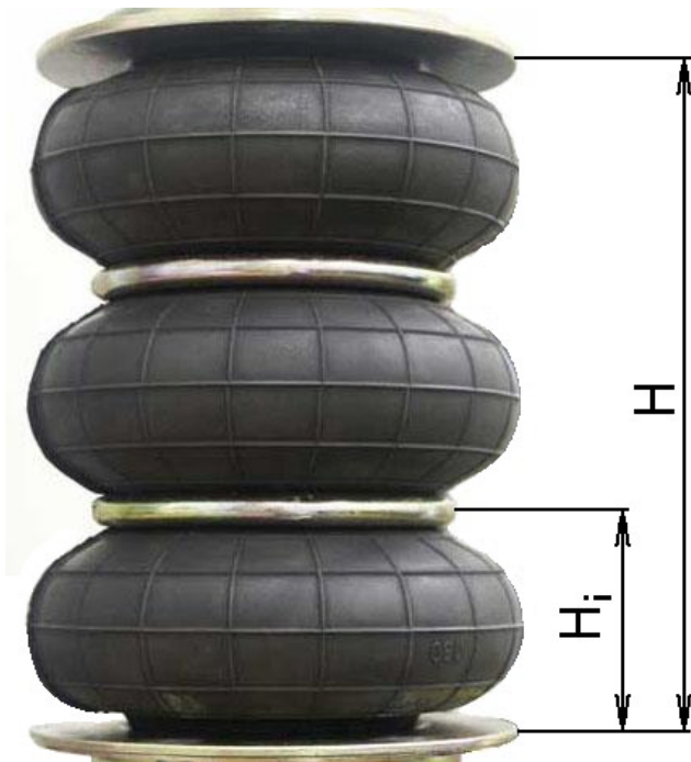
Figure 2 Design of the multi-bellows air spring; H-height of whole multi-BAS; H_i -height of one bellow of multi-BAS
