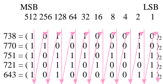
Figure 1. An example showing the bit-transforming.
