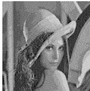
Fig. 6. The recovered image when 3 shares are received in the (r_1, r_2, r_3) = (3, 4, 5) case. The PSNR is 19.24 dB.
