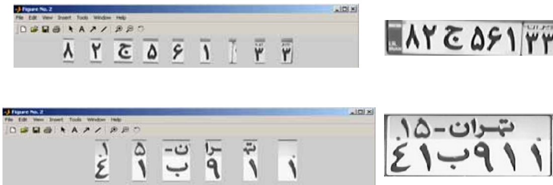
Figure 4. Result of program two kinds of iranian plate, (left) the result of program, (right) the image of plate
