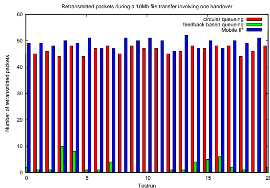
Figure 9: Number of retransmitted during a 10Mb file transfer.
