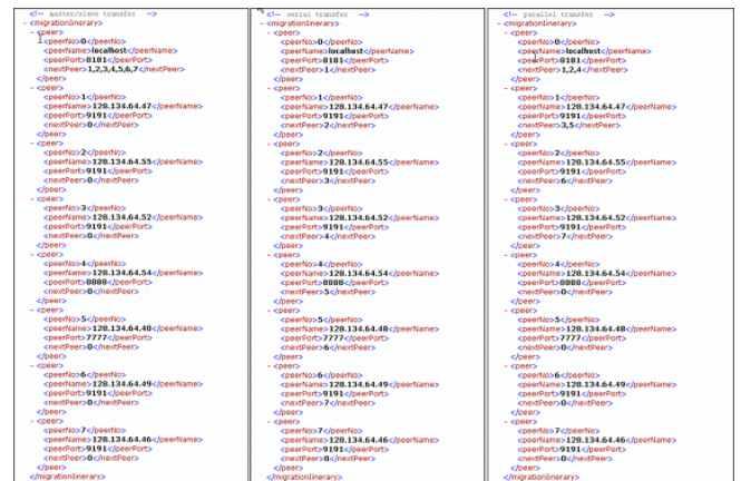
(a) master/slave type (b) serial type (c)parallel type Fig 8. Migration Itinerary
