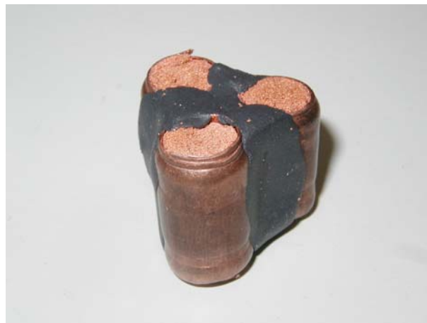
Fig. 3. Bundle of 3 - 2cm long sintered material filled pipe.
