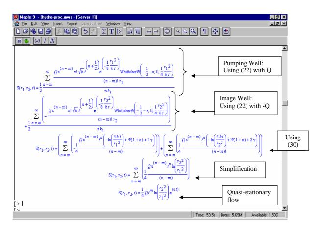
Figure 1. Total drawdown for a semi-infinite confined aquifer bounded by a river and with a well with pumping rate of the form (12). The method of image well is applied.
