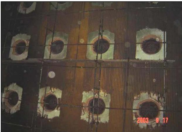
Fig.1 General Arrangement of Burners
