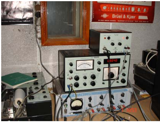
Fig. 7. Signal generator with amplifier Brüel&Kjaer 2706-1027
