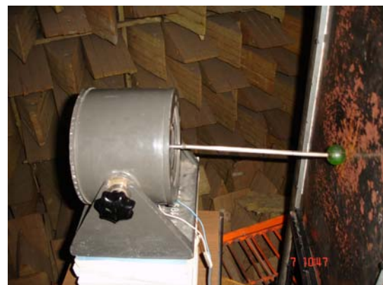
Fig. 6. Electro-magnetic hammer RFT 101.
