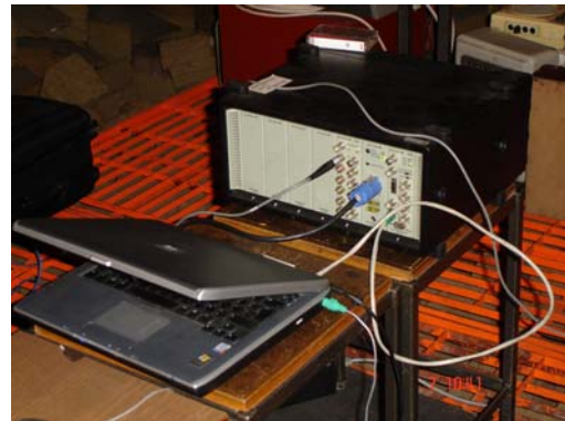
Fig. 5. Pulse system Bruel&Kjaer 3560D and Lap-Top HP.
