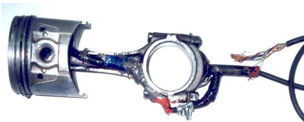
Figure 4. A suitable pass way for preventing wire entanglement around the crank angle
