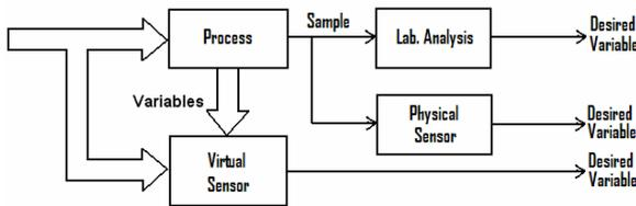
Figure 1. Virtual sensor illustration
