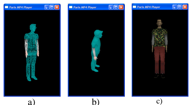
Figure 9 – Visualization by the rendering engine: a) in wireframe, b) in Goroud shaded and c) textured model.
