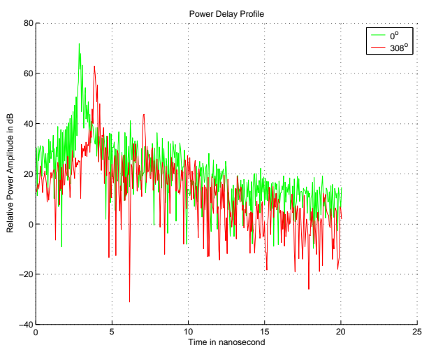
Figure 4: Power delay profile measured at desk pictured in Fig. 2. Note the delay and relative reduction of power of the signal received at 308 degrees in azimuth.
