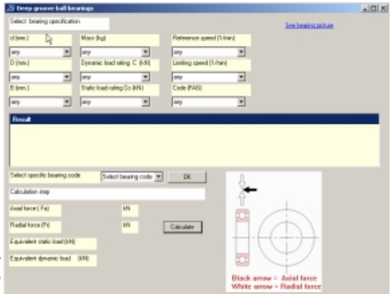
Fig.5. Example of program main window for bearing selection (deep groove ball bearings)
