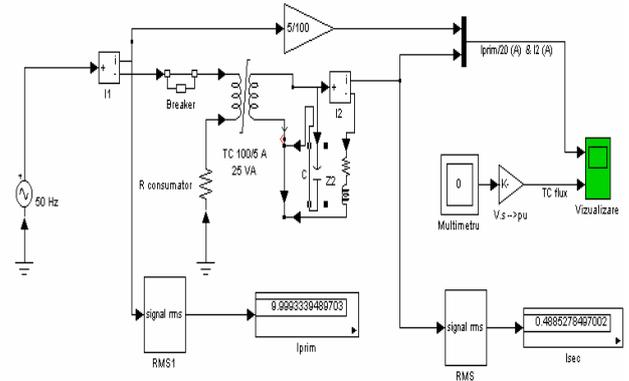
Fig. 10. SIMULINK model for passive compensation of current transformer.
