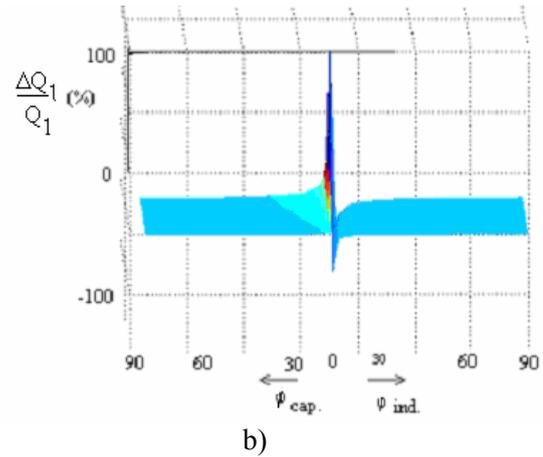
Fig. 1. Errors of measurement on the electrical power: a) active; b) reactive.
