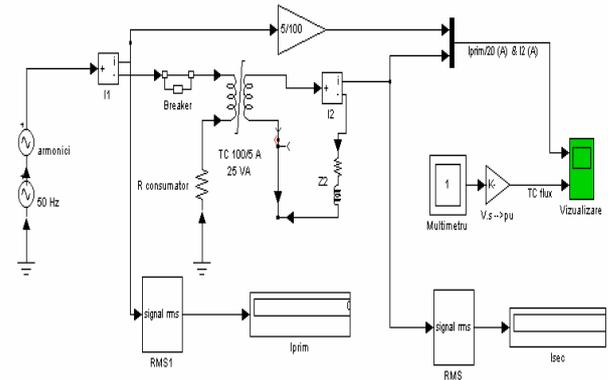
Fig. 2. SIMULINK model for the current transformer.
