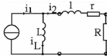
Fig. 6. Model of current transformer.
