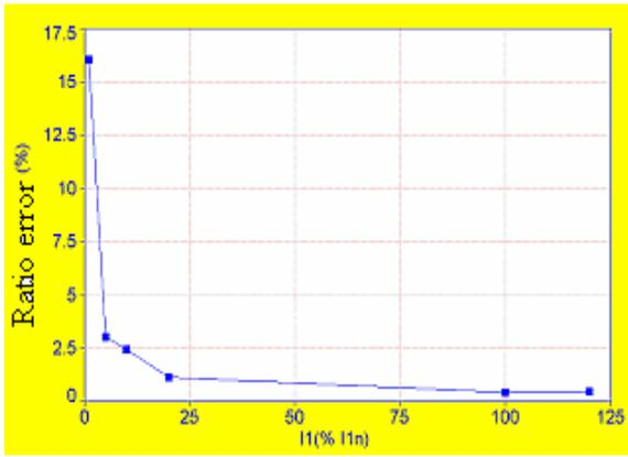
Fig. 3. Errors of the instrument transformer.
