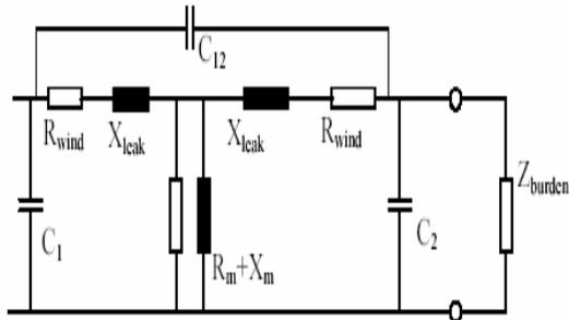
Fig. 4. Model for instrument transformer at medium frequencies.
