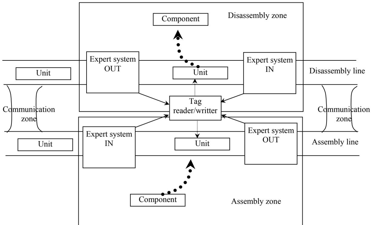
Fig.2. Systems integrated within a zone
