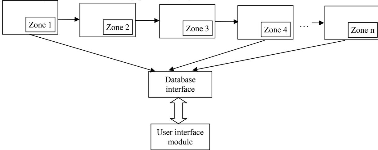
Fig.1. A model of a decentralized assembly line
