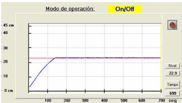
Figure 12. System Response using an On/Off controller
