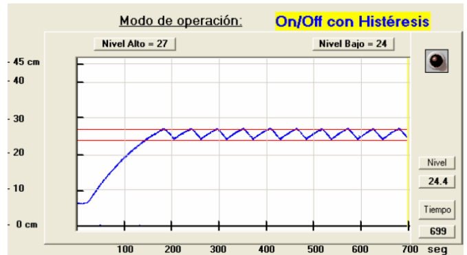
Figure 13. System Response using an On/Off controller with hysteresis
