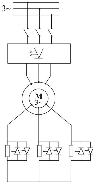
Fig.4 – Speed adjustment of the asynchronous motor using individual static contacts
