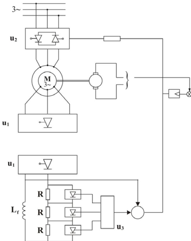
Fig.2 – Block diagram of the electric drive system for an asynchronous power motor with coil rotor
