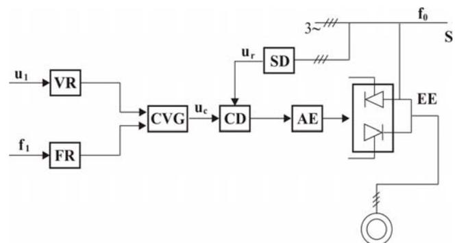
Fig. 1 – Flow chart of the electric drive system by frequency converter for asynchronous motor
