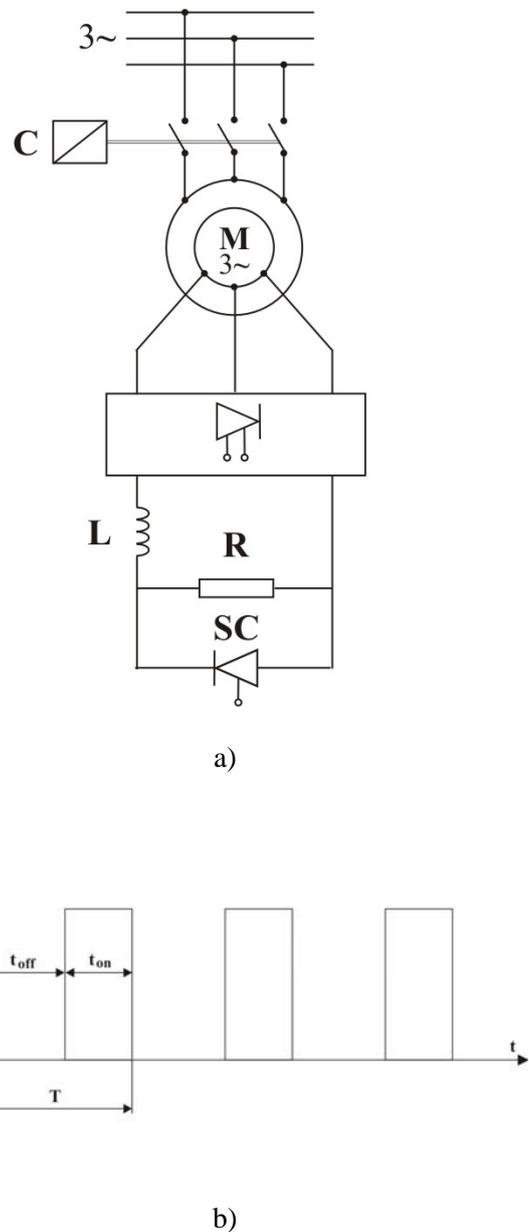
Fig.3 – System for adjustment speed to asynchronous motor using the method of rotor flux bearing
