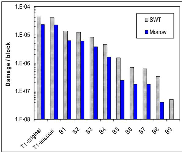
Fig. 5. Damage distribution for the original signal, the mission signal and bump segments (B1-B9 are the bump numbers, as shown in Fig. 4c)
