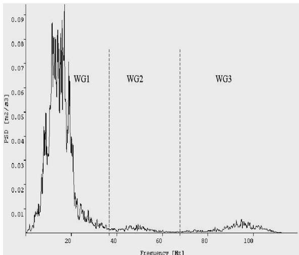
Fig. 2. A PSD plot showing the dividing of a frequency spectrum into three wavelet group (WG)
