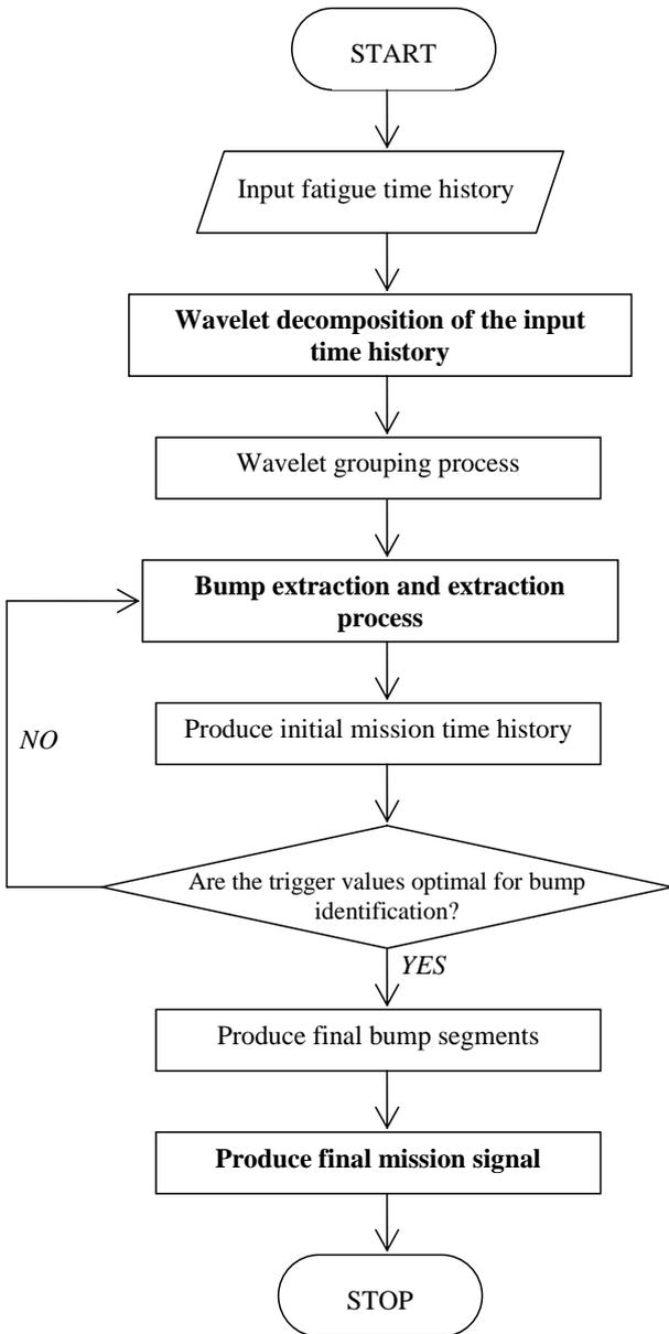
Fig. 1. Flowchart of the WBE algorithm.
