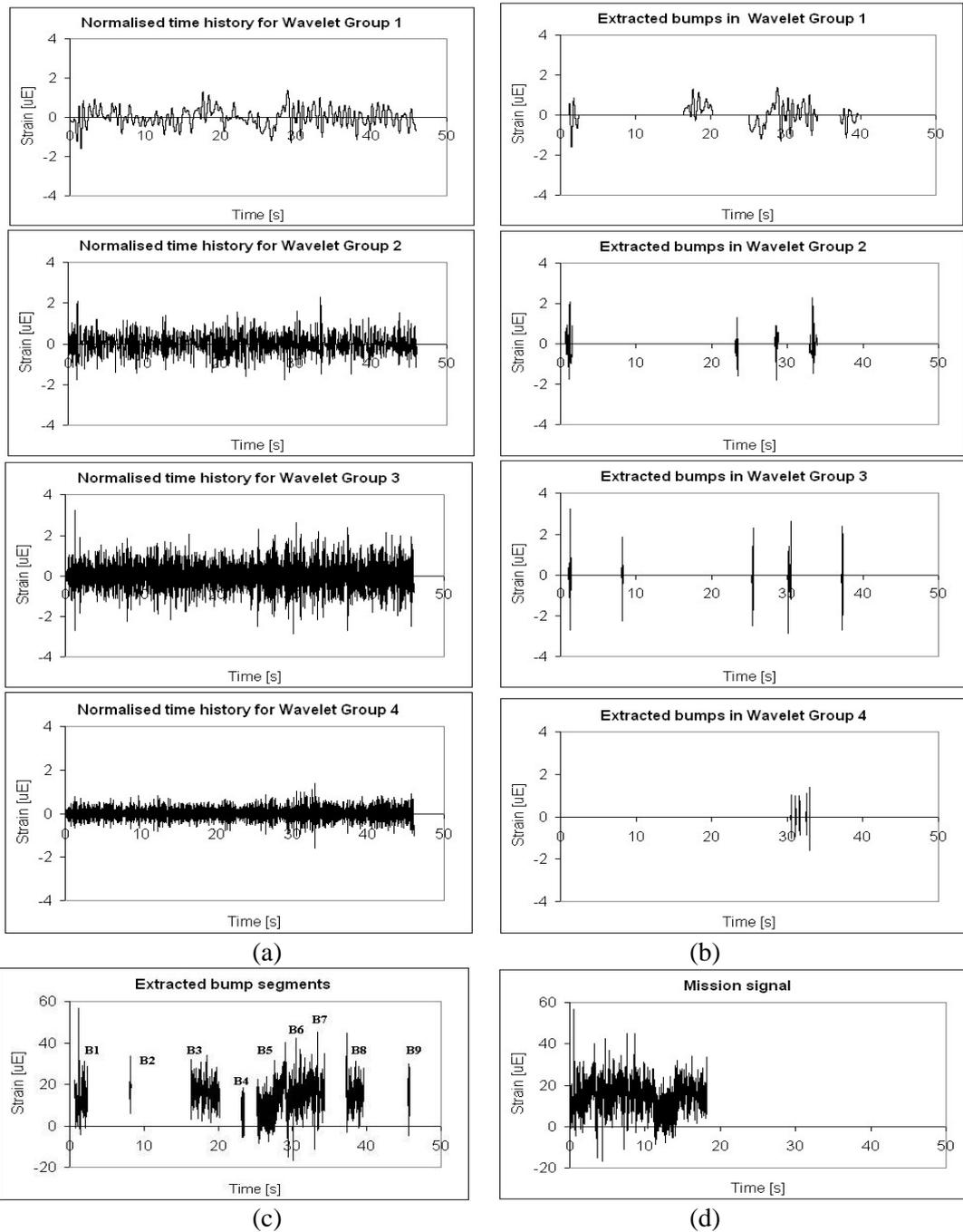
Fig. 4. Normalised time history for all wavelet groups (b) Location of bumps in all wavelet groups, (c) The extracted bump segments (in original scale) at their original location of the input fatigue signal, (d) The mission signal
