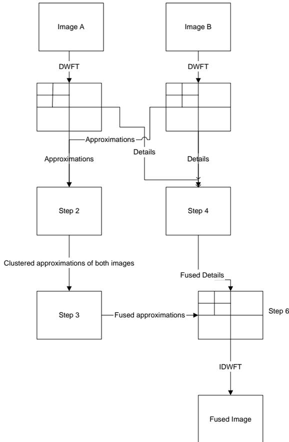
Figure -1 Flowchart of Proposed Algorithm
