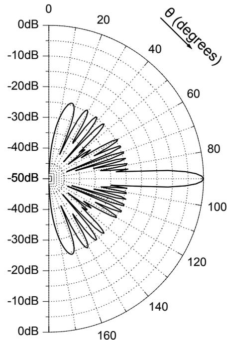
**Fig.4: Radiation pattern of an optimized broadside antenna array of 20 collinear wire dipoles.**
