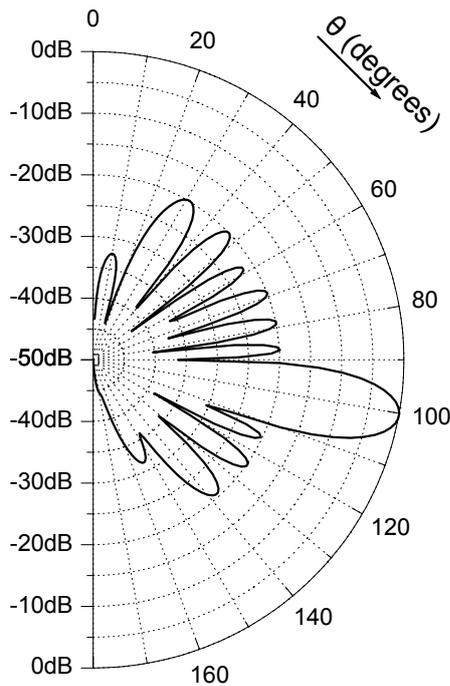
**Fig.6: Radiation pattern of an optimized antenna array of 10 collinear wire dipoles with main lobe direction at  $\theta=100^\circ$ .**
