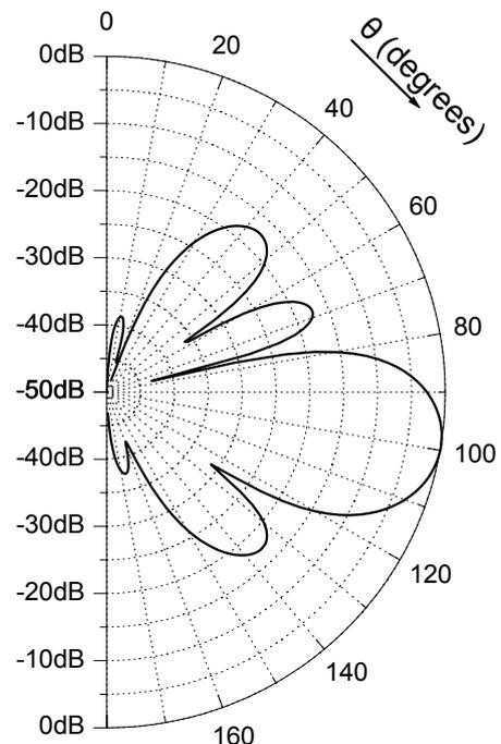
**Fig.5: Radiation pattern of an optimized antenna array of 5 collinear wire dipoles with main lobe direction at  $\theta=100^\circ$ .**
