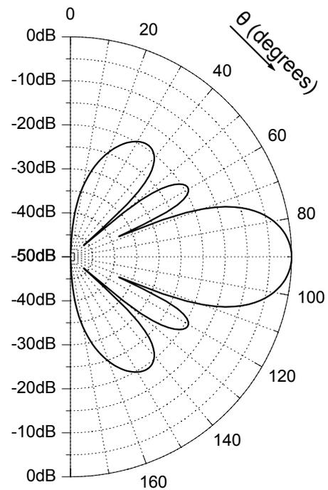
**Fig.2: Radiation pattern of an optimized broadside antenna array of 5 collinear wire dipoles.**
