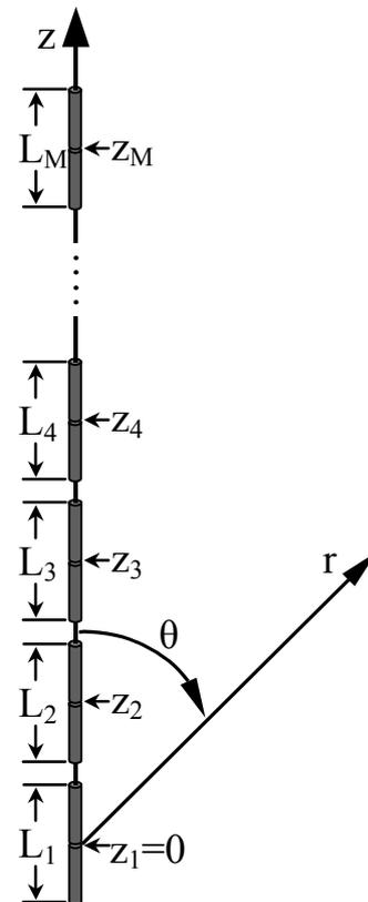
Fig.1: Collinear wire-dipole antenna array.
