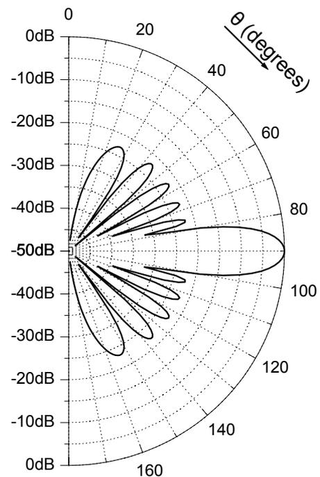
**Fig.3: Radiation pattern of an optimized broadside antenna array of 10 collinear wire dipoles.**
