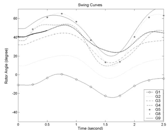
Figure. 2 Swing curves of all generators in the external system
