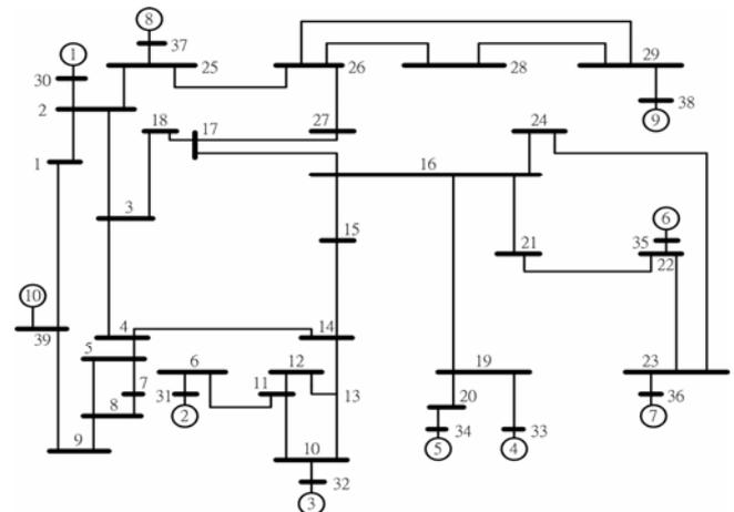
Figure. 1 One-line diagram of the New England test system
