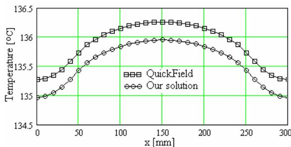
Fig. 15 Temperature distribution ( $y = 0$ )
