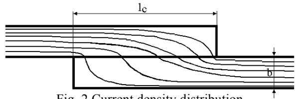
Fig. 2 Current density distribution
