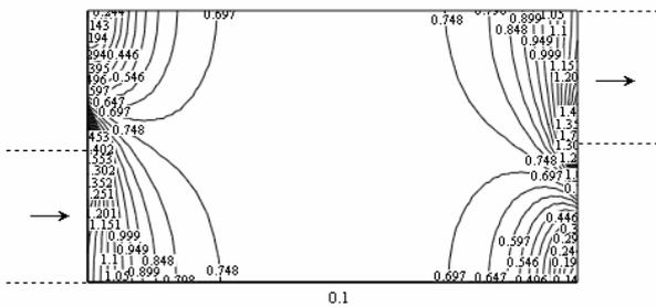
Fig. 6 Current density distribution in the contact region (in  $A/mm^2$ )
