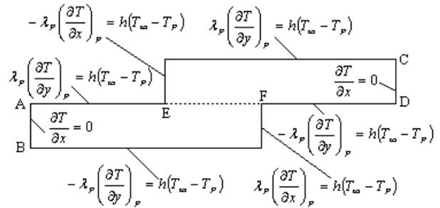
Fig. 4 Analysis domain and boundary conditions for thermal model
