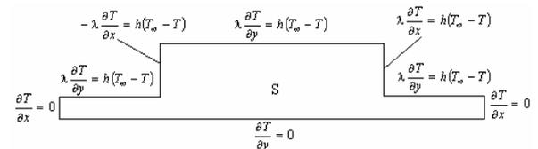
Fig. 10 Thermal model for numerical validation
