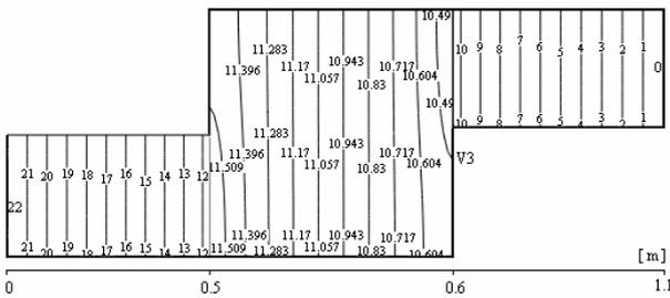
Fig. 5 Potentiel distribution (in mV)
