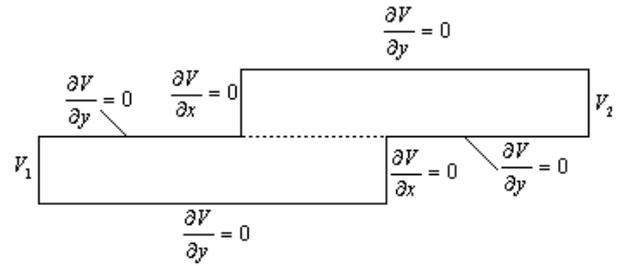
Fig. 3 Analysis domain and boundary conditions for electrical model
