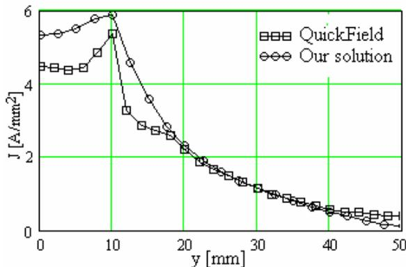
Fig. 14 Current density distribution ( $x = 55 \text{ mm}$ )
