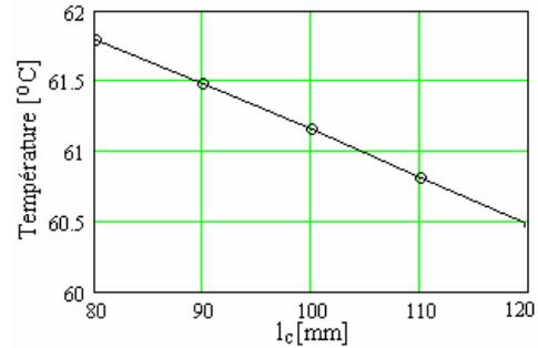
Fig. 8 Maximum temperature of contact versus length of contact ( $S_c = 1.01 \text{ kW}$ ).
