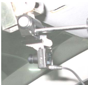
Fig. 1 The monochromatic CCD mounted behind the windshield
