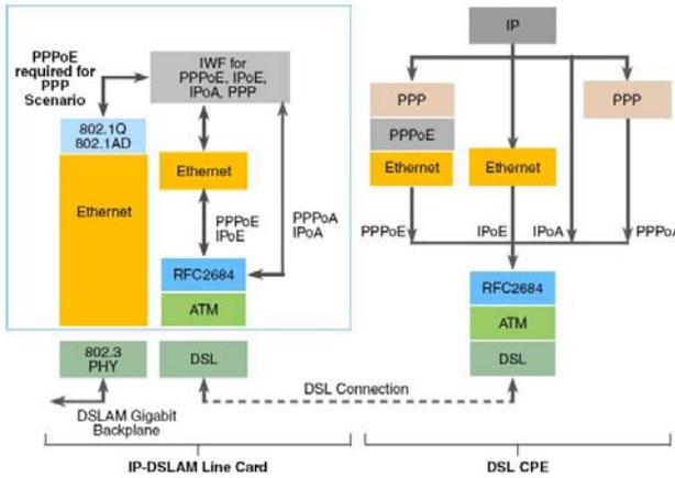
Fig. 3 Typical connection between IP-DSLAM and CPE
