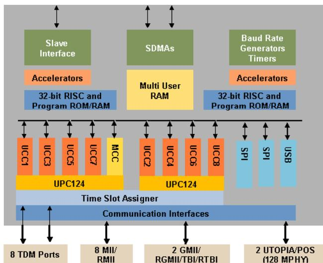
Fig. 1 QUICC Engine™ coprocessor block diagram
