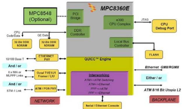
Fig. 2 Typical NodeB NIC implementation with MPC8360E
