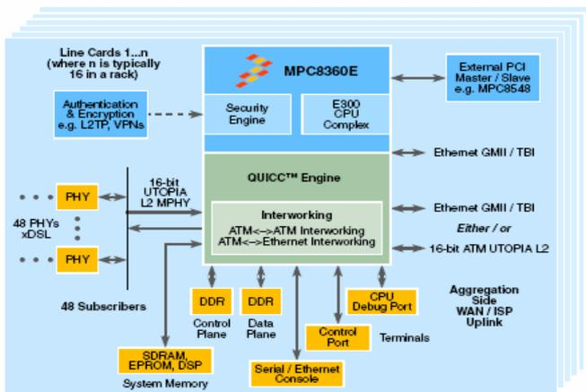
Fig. 4 Typical IP-DSLAM implementation with MPC8360E
