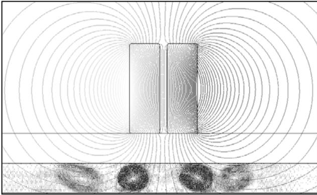
**Figure 10** Fluid velocity field with magnetic potential
